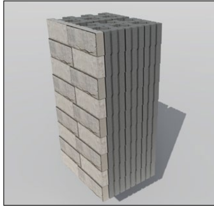
Diagram 15—3 deep. Maximum height of 5½ feet
