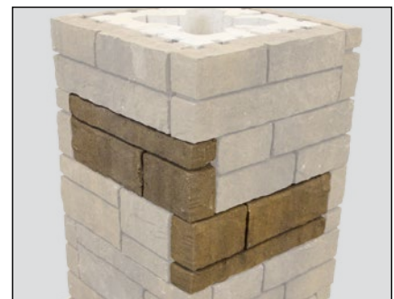
Diagram 25—Stagger veneers to break up lines
